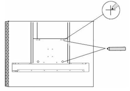
2) Position the hood against the wall that you are intending to install it on and mark the position of the support holes that are to be drilled (as shown in the figure below).
