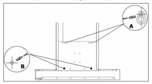
2a) The support screw holes are indicated by figure A in this drawing and the anchoring screw holes are indicated by figure B.
