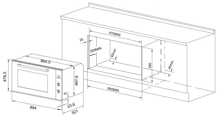
The panels of the adjacent cabinets must be made of heat-resistant material .In particular ,cabinets with a veneer exterior must be assembled with glues which can withstand temperatures of up to 100°C.
