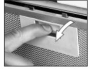
**1)** Remove the metal grease filters.
