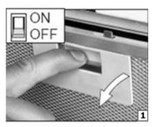
1) Remove the grease filters.
